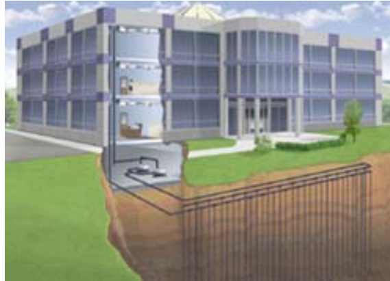
Figure 4.1.5 Geothermal Heat Pump with a Vertical Water Loop (Picture Courtesy of McQuay Corporation)
